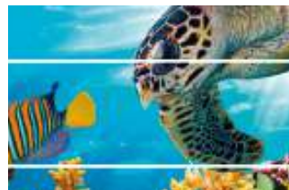
Gap/White streaks (Excessive feeding amount)
