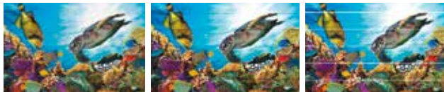
Incorrect bi-directional drop landing position
